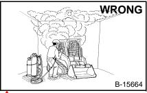
Have good ventilation when welding or grinding painted parts. Wear dust mask when grin in painted parts. Toxic dust and grant can be produced.
