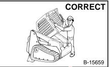
Use the correct projective to lift or lower operator car.
