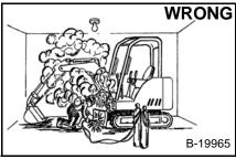
Have good ventilation wher welding or grinding painted it rts Wear dust mask when grind g painted parts. Toxic dust 2 can be produced.
