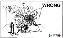
Have good ventilation when welding or grinding painted, retained when grinding painted parts. Toxic dust and gas can be produced.
