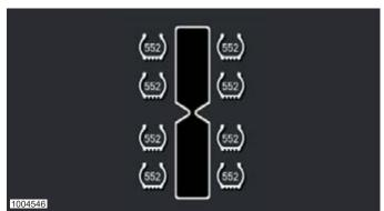
The top of the screen represents the front of the machine based on which direction the seat is facing. When the seat rotates, the tire display adjusts so that the tires in front of the operator always display at the top of the screen.
