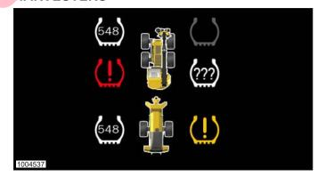
The top of the screen represents the front of the machine. The number and position of tires shown varies by machine configuration. The machine icon can be used as reference for tire location.
