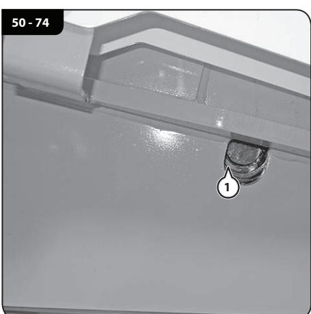
Remove the circlips on the left of the telescopic boom cylinder base pin (1, [50 - 74](#)).
